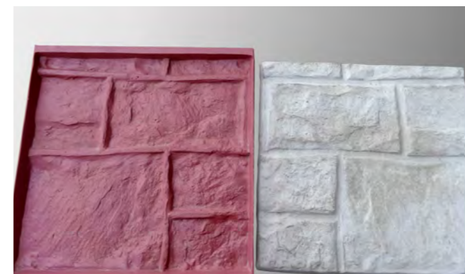
Cavity made with GM 965-55, concrete casting
