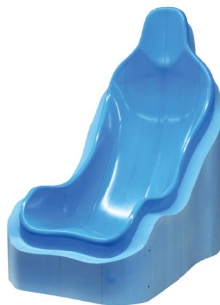
Master model for racing seat tool made of eboard EP 138
