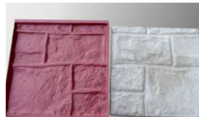
Cavity made with GM 965-55, concrete casting
