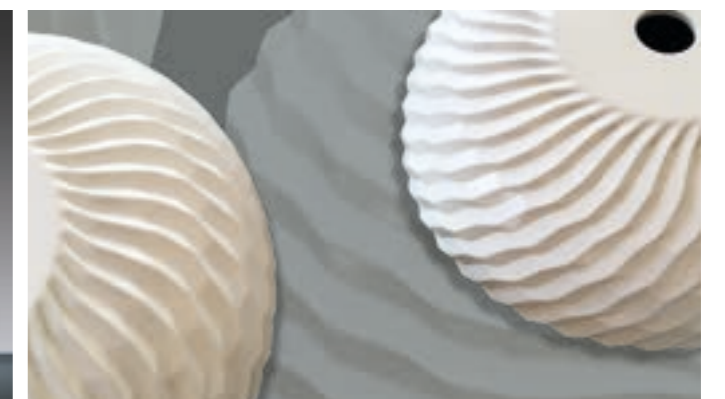
3D-printed sink infiltrated with ebalta resin IH 16
