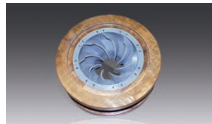
Core box made with GH 760
