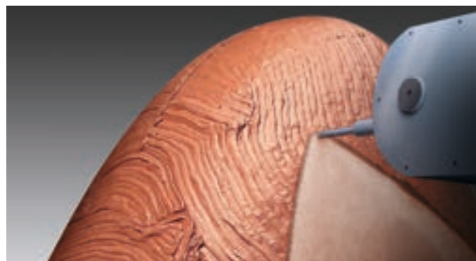
Milling of lay-up paste P 26
