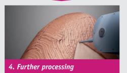
Depending on the mould size, application of the paste is finished within 1-2 days, afterwards the model can be machined and painted.
