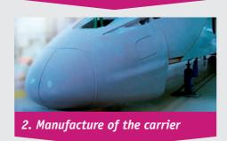
Depending on your requirements, and whether being of polystyrene, polyurethane foam or laminate, our partners manufacture the carrier in short time.
