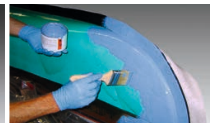
Application of gel coat OH 6-1
