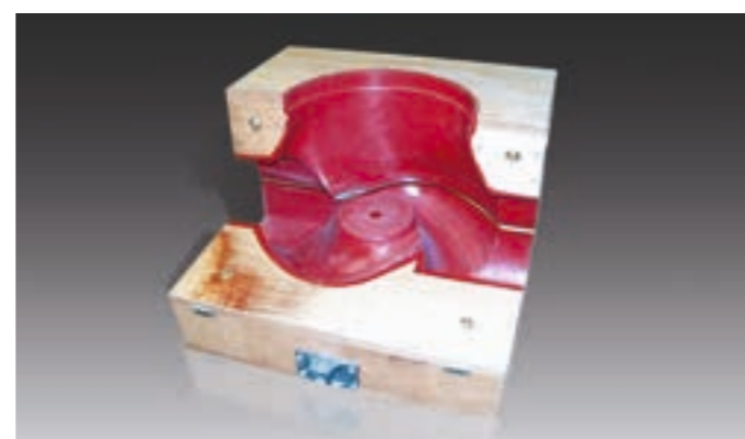
Core box made of OH 11 with PS 03-1
