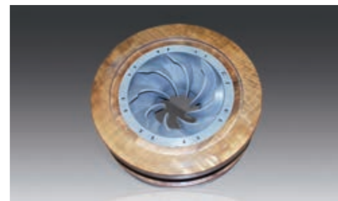
Core box made of GH 760
