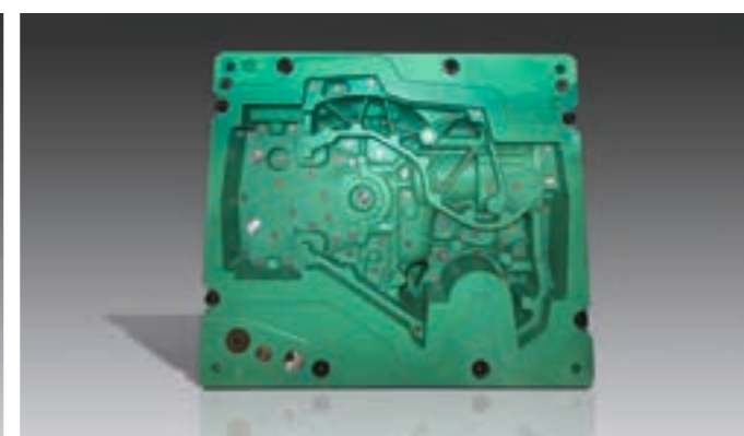
Core box made of ebaboard PW 920
