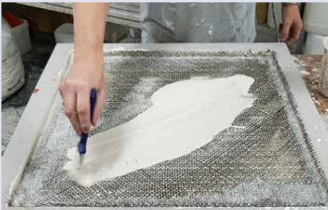
To laminate, you have to work wet in wet. A quick way to apply A1 is with a brush or roller.
