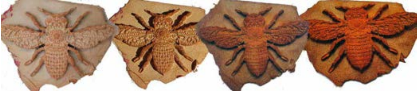
After exposure to water, the Iron powder mixed into the A1 gives beautiful natural and unique rust effects.
