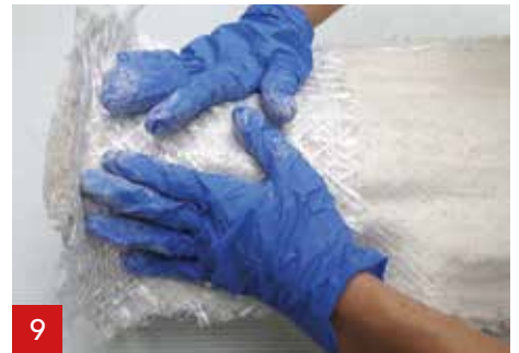
6 Add the A1 Triaxial fibre on the wet A1. Continue until the entire silicone mould is covered with A1 and a layer of A1 Triaxial fibre.
